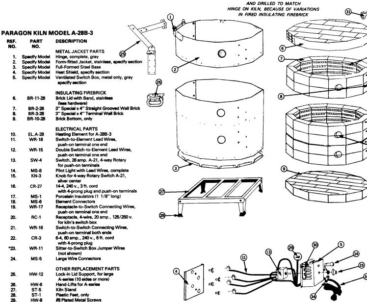
\*Only for kilns equipped with kiln sitter.
