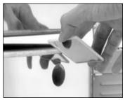
With a mirror, you can detect moisture escaping from the kiln. Keep the lid in the vented position until the mirror no longer fogs.
