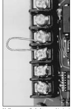
Half a paper clip being used to test the thermocouple circuit on the controller.
