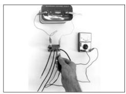
Testing a relay with a 12 volt lantern battery.
