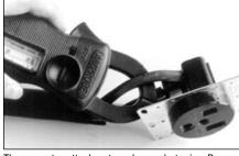
The ammeter attaches to only one hot wire. Be sure breaker is shut off before you remove the receptacle cover.
