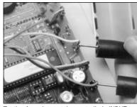
Testing for voltage at the controller's INPUT terminals.
