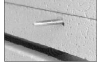
The 1/8" thermocouple should protrude into the firing chamber ½" - 5/8". The ¼" thermocouple should protrude 1" into firing chamber.
