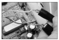
Use alligator clips to test for voltage at the disconnected INPUT wires.
