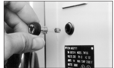
The fuse holder is on the side of most kiln switch boxes. Even if the wire in the fuse looks okay, the fuse could still be bad. Check with an ohmmeter.
