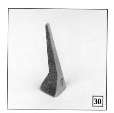
Witness Cones: One is placed inside the kiln on the hearth plate (as close to the center as possible) for each firing. Duncan recommends the Orton Self-Supporting Large Cone for your kiln.
