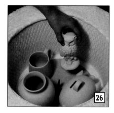
Loading your kiln properly helps ensure a good, fully mature firing (photo 26).
