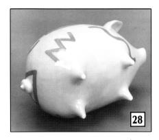
When firing porcelain greenware pieces with lids, fire them assembled and apply a generous dusting of alumina hydrate to one surface of any areas that touch. This will prevent the pieces from fusing together.
