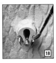
2. Apply a coating of kiln wash to the top of the cone supports and the bottom of the sensing rod, unless already done. (See Chapter 2, steps 5 and 6.) (photo 18).
