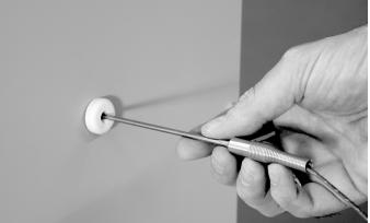
The porcelain insulator that is furnished with the controller is used to mount the thermocouple in a ½" hole on the kiln. Do not allow the thermocouple to fall out of the kiln during firing, or the kiln could overfire.
