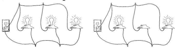
The second type of circuit is the parallel circuit. In this type, electricity flows to each light bulb without having to flow through the others. If one bulb burns out, the other bulbs continue to work.
