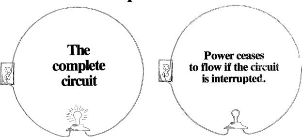
When electricity flows from its source, such as 120 volt house current, to light a light bulb, it must also return to its source. Electricity must flow in an unbroken circuit. If the circuit is broken, electricity stops flowing. Every time you turn on a wall switch, you are completing the electric circuit to a light bulb. When you turn the switch off, you are interrupting the circuit.
