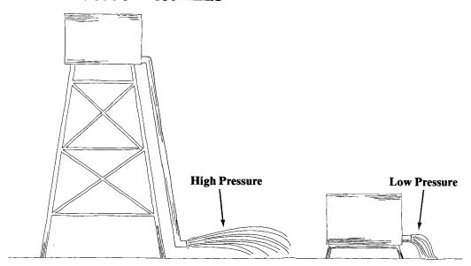
There are two water tanks. One is at ground level, and the other is several hundred feet high. By connecting a pipe of equal size to each tank and letting the water run out, we can see that the high tank has much more water pressure than the low tank. The high tank will be empty much sooner. The higher the water tank, the harder will its water come pounding out of a pipe. Gravity increases water pressure with altitude.
