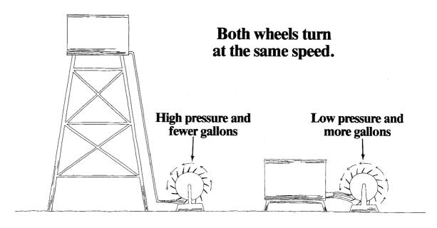
There is a way to make both wheels turn at the same speed. We remove the pipes and replace them with a small diameter pipe and a large diameter pipe. The small pipe is hooked up to the high tank and the large pipe to the low tank.
