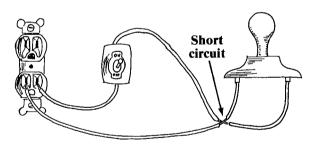
Damaged insulation on wire exposes bare wire, resulting in short circuits. In the circuit above, two bare wires have touched each other. This contact allows the electricity to complete the circuit without going through the light bulb. It bypasses the light bulb. Because the light bulb is no longer part of the circuit, the current flows with very little resistance, and it can melt the wires. But if a fuse is in the circuit, the fuse will melt before the wire can overheat.
