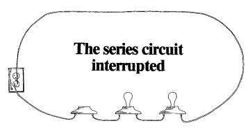
If one bulb in the series circuit is removed, the other two light bulbs will no longer work. Removing a bulb puts a gap in the circuit so that current can no longer return to its source. If a switch is added to the series circuit, the switch turns off all the light bulbs. You cannot have one bulb on and the others off. They are either all on or all off.
