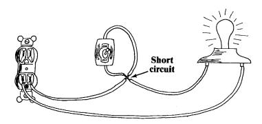
In the circuit above, bare wires have touched near the switch. Current then flows past the switch, so the switch is no longer part of the circuit. The light bulb stays on all the time whether the switch is on or not. But since the light bulb is still in the circuit, the wire does not overheat. The resistance (ohms) of the light bulb prevents too many amps from flowing through the circuit.
