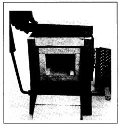
Lift out the roof firebricks. Be careful not to disturb the thermocouple.
