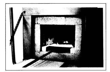
can place a blade in each space between the pins and fill up the knifeholder. The upright pins separate the knives so they will heat evenly.
