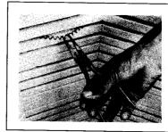
3 As the element shrinks, work it back toward the groove and into place. Work rapidly, and at the first sign of stiffness in the coils, stop bending and reheat the
