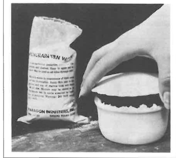
High fire kiln wash will keep porcelain greenware that must be fired together from sticking. The kiln wash should be dry; wet kiln wash is difficult to remove after firing.
