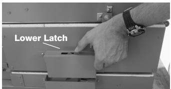
To raise the kiln body, press the lower latch forward. That releases the kiln so it can separate from the bottom.
