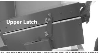
As you raise the kiln body, the upper latch should automatically engage the latch pin. The latch keeps the lid closed when the kiln is raised.
