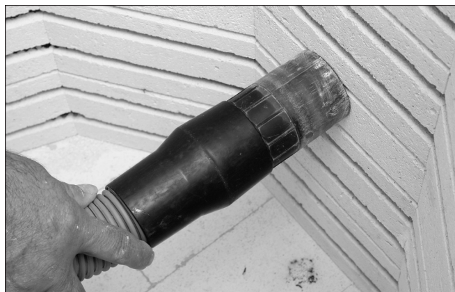
Place the vacuum hose directly over the Kiln Sitter tube.
