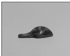
An overfired witness cone.
