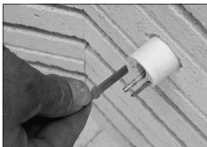
Remove the cone supports before vacuuming the Kiln Sitter tube.
