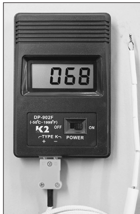
A pyrometer measures the heat inside a kiln.
