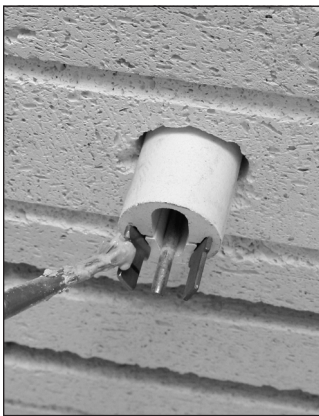
Apply kiln wash to the cone supports. Let the kiln wash dry before inserting the cone.
