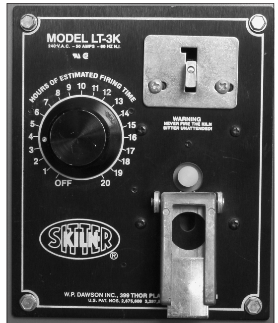
The Kiln Sitter with the weight in the lowered position.
