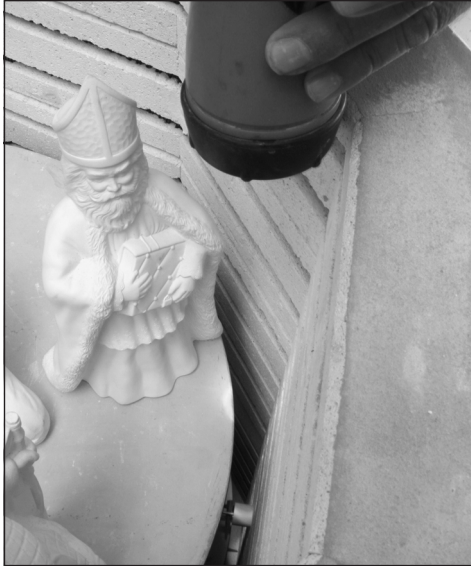
Check the Kiln Sitter cone with a flash light before closing the lid and firing the kiln.
