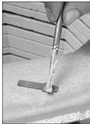
Applying the kiln wash is easier if you remove the cone supports.
