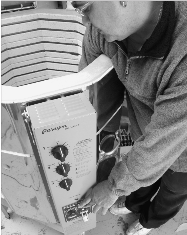
Loading a cone into the Kiln Sitter requires two hands or a helper.
