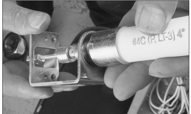
Align the notch on the new Dawson tube assembly with the pin on the bracket. This assures that the porcelain tube slot will be perfectly vertical inside the kiln.
