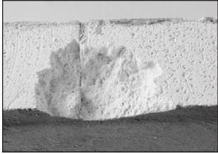
Use this technique to repair wall damage where the lid touches the kiln wall.
