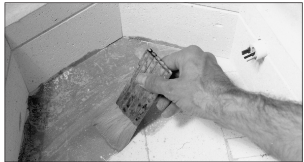
Coat the firebrick floor with kiln wash or glass separator. If your kiln has sidewall elements, hold a piece of cardboard in front of the elements to protect them from contact with kiln wash.
