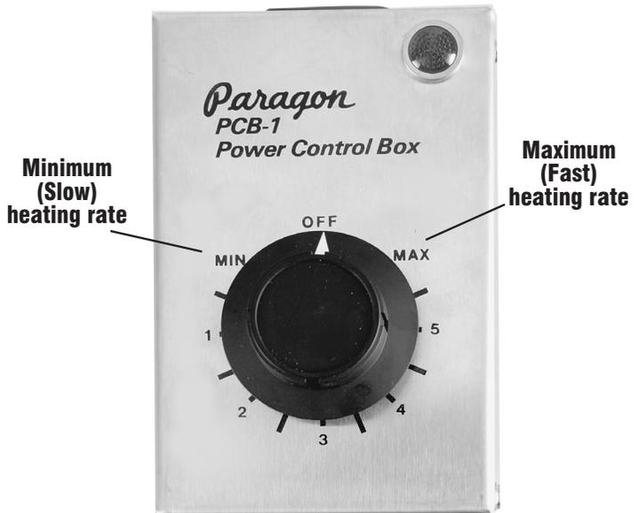
control the heating rate. When the switch is turned to Max (maximum), the clicking noise ceases, because the power remains on continuously.
