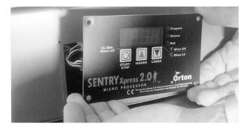
**2** Remove the four screws that hold the controller to the kiln. Carefully remove the controller from the kiln. Leave wires attached to the controller.
