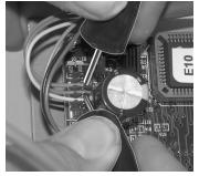
facing you. Plug the kiln back in. Touch voltmeter probes (in AC mode) to both INPUT connections (the white and orange wires).
