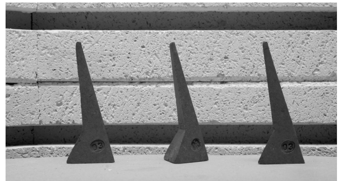
The heating element in the background should be lined up with the lower part of the witness cones. If the element is too high, the tips of the cones will disappear from view when they bend.
