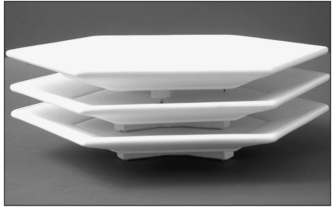
Separate horizontally stacked china painted plates with stilts. Do not stilt soft-bodied ware such as bone china.
