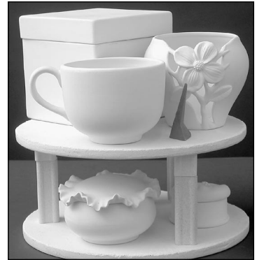
Group similar sizes of ware together. Place taller pieces on the top shelf. Line up posts vertically.
