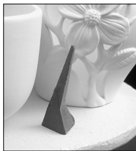
Position the cone so that it will not touch nearby ware when it bends.
