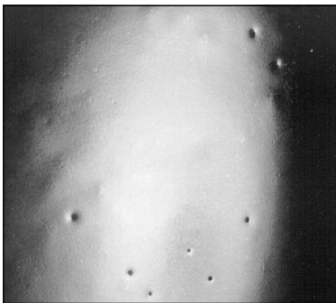
Pinholes from underfired bisque.
