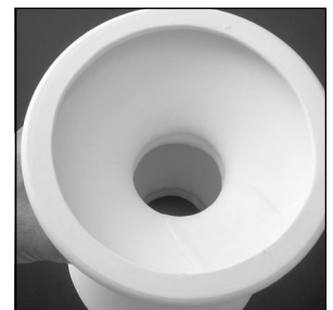
Slip-cast ware is hollow. If the clay is solid and very thick, it will break in the kiln.
