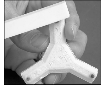
Cleaning stilt wire with a stilt stone.
