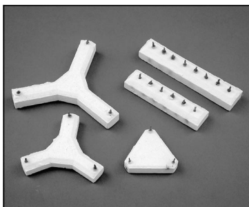
Use stilts to separate the ware from the kiln shelf.
