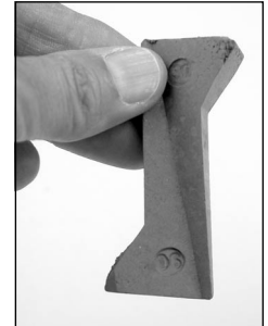
Self-supporting cones must be broken apart before use. Note that the cone number is stamped on the base.
