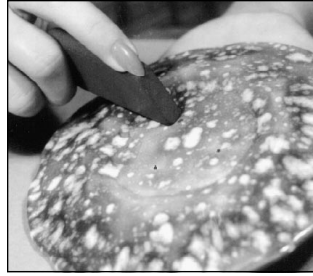
Removing stilt marks with a stilt stone.
