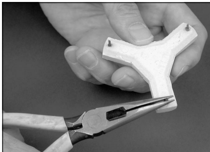
Straightening a stilt point.
