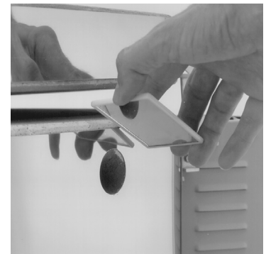
Vent the kiln until moisture no longer fogs a mirror.
