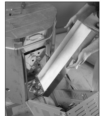
On some kilns, the element cover must be removed to gain access to the thermocouple.
