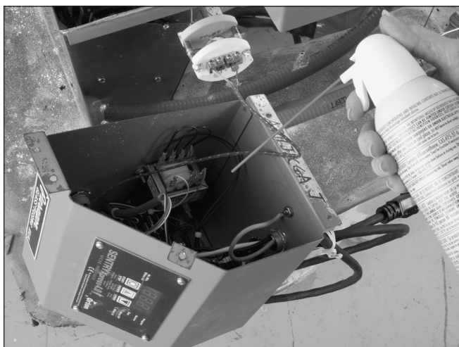
Whenever you open the switch box, blow out the dust with canned air.
