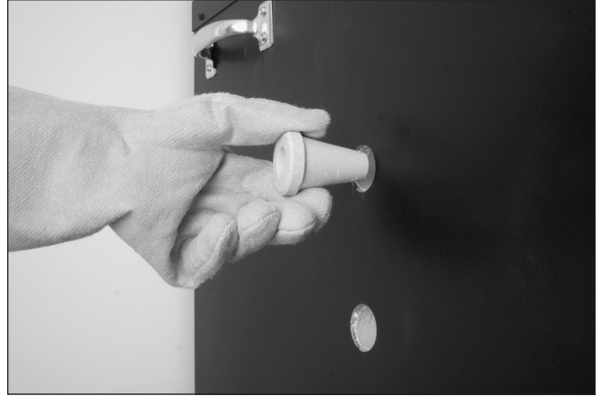
Remove the peephole plug to vent the kiln.
