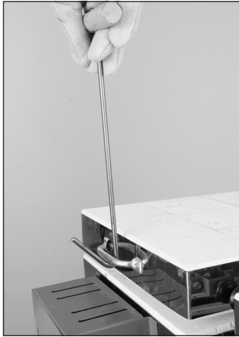
At the end of the venting period, remove the post with a Lid Lifter and hot glove (available from Paragon).
