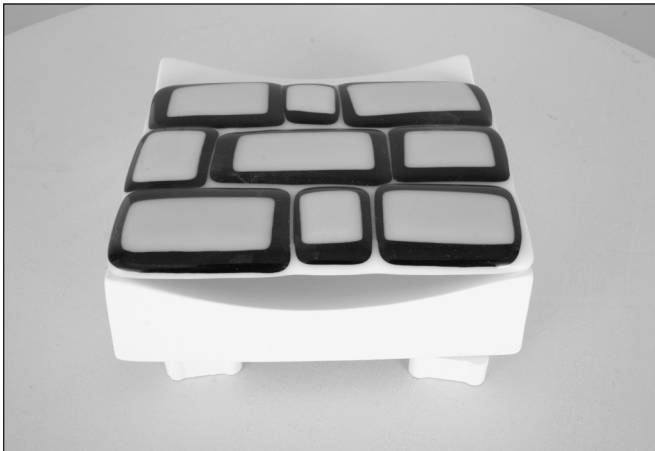
Separate a sagging mold and kiln shelf with 1/2" (12.5 mm) high posts.
