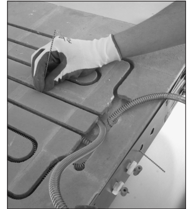
Use a section of the old element pigtail to guide the new element pigtail into the hole. Note that the porcelain insulator goes in the outer side of the hole.
