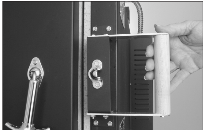
Open the door about ¼" (6.35 mm) to vent a front-loading kiln.
