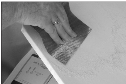
You can also remove loose kiln wash with grit cloth and then apply a new coat.
