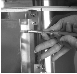
Removing the element cover to gain access to the element connectors. Not all kilns have an element cover.
