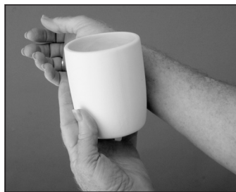
Greenware that feels cool against the wrist still contains moisture.
