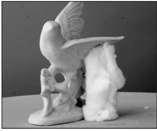
You can support delicate porcelain with wads of ceramic fiber.
