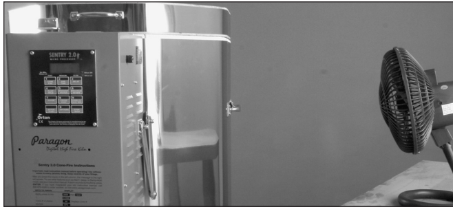
A small 4" diameter fan can reduce cooling time by 1 ½ hours.
