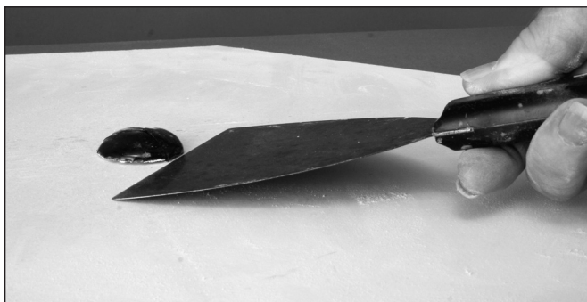
Hold the putty knife at a sharp angle to remove glaze from a shelf.
