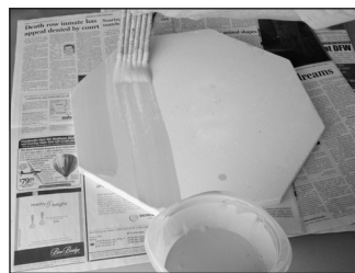
Kiln wash protects shelves and the kiln's brick bottom from drops of hot glaze.
