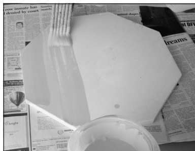
Applying kiln wash with a haik brush.
