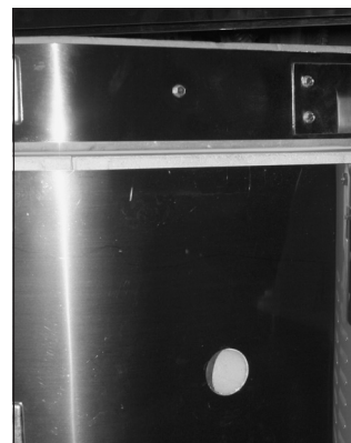
The light around the edge of the lid and inside the peephole changes color as the kiln gets hotter. You can learn to estimate temperature by the color of that light.
