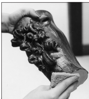
To “dry foot” a piece, remove all glaze from the portion of the piece that will rest on the shelf.
