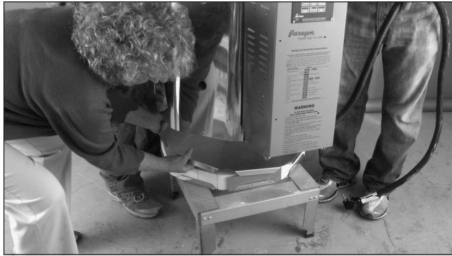
Place the new base plate on top of the brick bottom while your helpers hold up the kiln.
