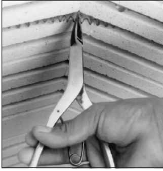
Expanding coils with automotive snap-ring pliers.
