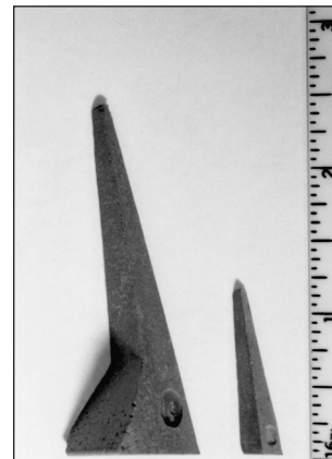
A self-supporting cone next to a small Kiln Sitter cone.
