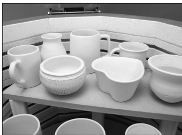
Have at least one element groove between the top shelf and the top of the kiln.
