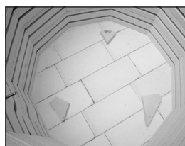
You can support the bottom shelf with small shelf pieces.
