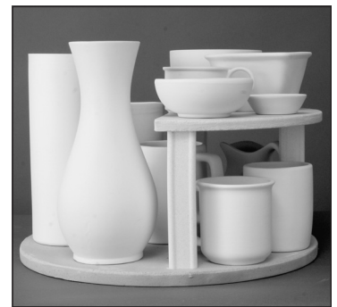
Use half shelves to load layers of ware next to tall pieces.
