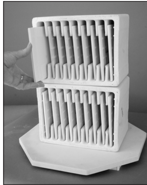
Tile setters conserve space inside the kiln when firing tiles.
