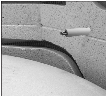
Keep ware and shelves at least 1" away from the thermocouple.
