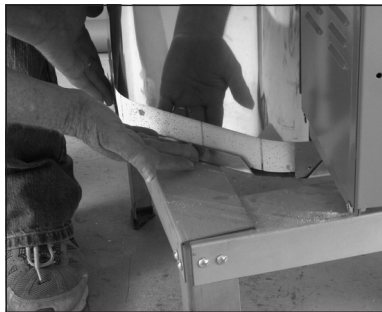
Slide the tabs on the new base plate under the stainless steel case.
