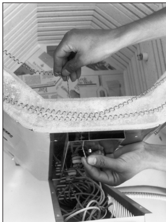
Arranging the element so it doesn't tangle up as you install it.
