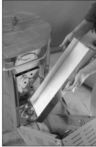
Removing the element cover to gain access to the element connectors. Not all kilns have an element cover.
