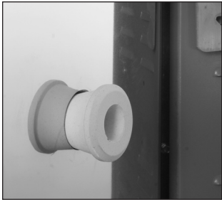
Keep the peephole plugs inserted if your kiln has a motorized downdraft vent.
