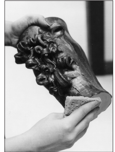
To dry foot a piece, remove all glaze from the portion of the piece that will rest on the shelf.
