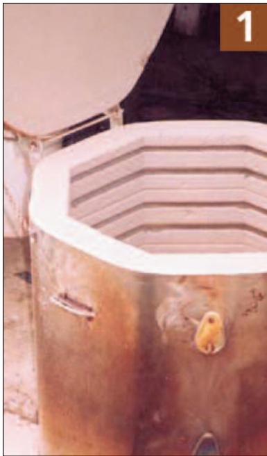
STEP 1 Take an electric kiln completely apart, and remove all elements, wires and switches. Drill a 1/4-inch hole in the center of the top and bottom (not shown).
