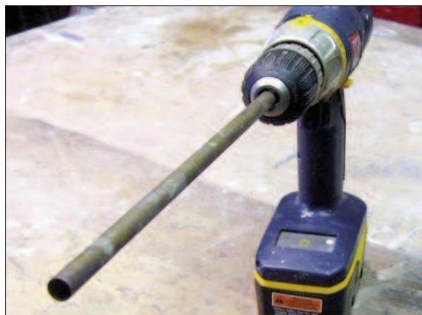
Copper tubing makes a great IFB drill bit.
