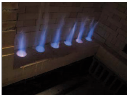
Two inches of water column.
