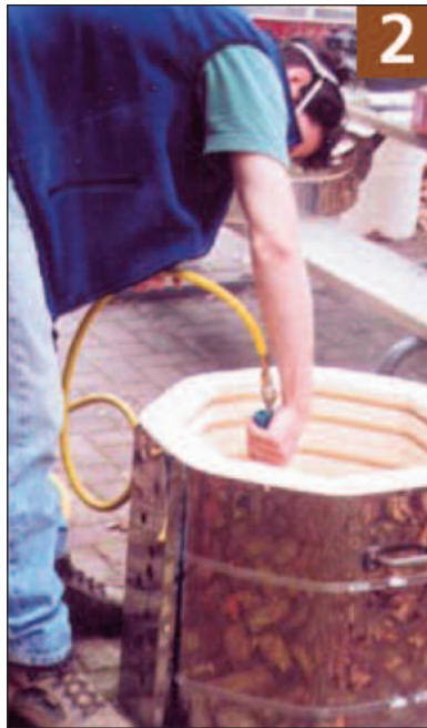
STEP 2 Thoroughly clean the kiln. While a vacuum cleaner works, using compressed air does a great job, but because of the dust, work outside and wear a mask.
