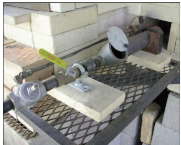
Bill's homemade burner system.
