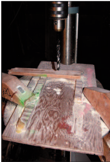
Construct a wooden template and clamp it to your drill press.
