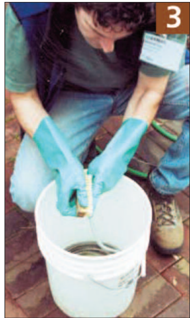
STEP 3 New elements have a thin manufacturing film on them so clean them well in household bleach using a small brush. Rinse them well and hang to dry.
