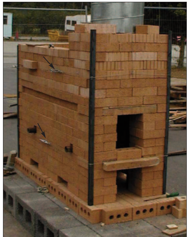
Look for the 2 tensioners/turnbuckles on the left-hand side of the kiln.
