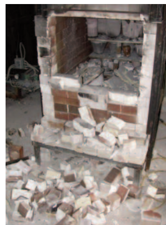
This is Nils Lou's small kiln that exploded because of a damp Advancer shelf. A student mistakenly washed an Advancer in water and let it soak to clean it.
