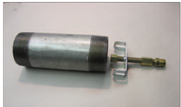
A simple homemade burner.
