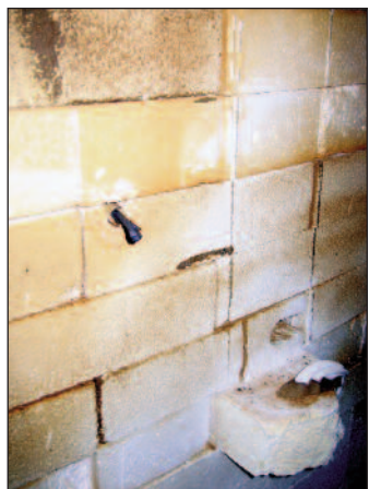
Placement of thermocouple in kiln.
