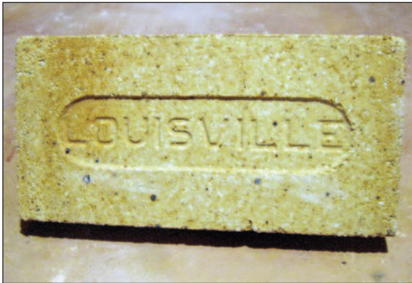
Hard brick absorbs more heat than insulating firebrick.
