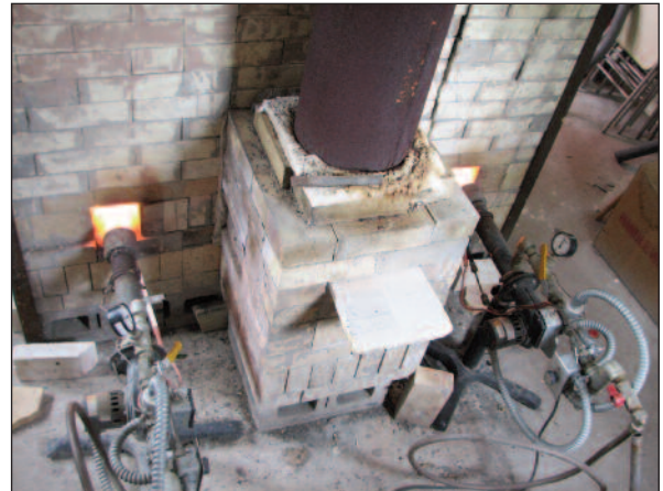
Tom Wirt and Betsy Price run Mark Ward power burners with power-out solenoids and thermocouples.
