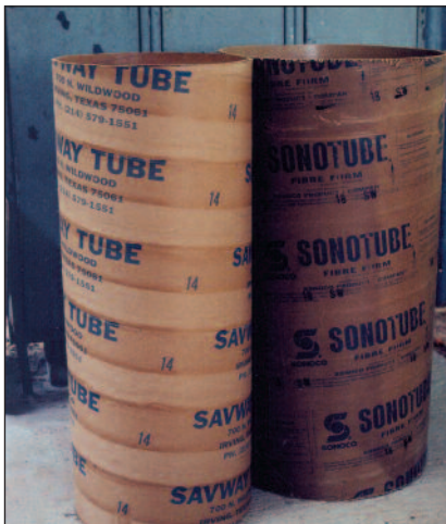
Two sizes of cardboard concrete forms are cut to the same length.
