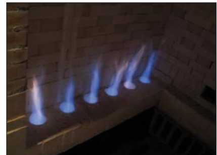
One inch of water column.
