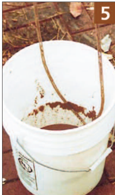
STEP 5 Thoroughly coat the coils by dipping them. Use a sheetrock mud pan or a 5-gallon bucket. Hang the coils up to dry.
