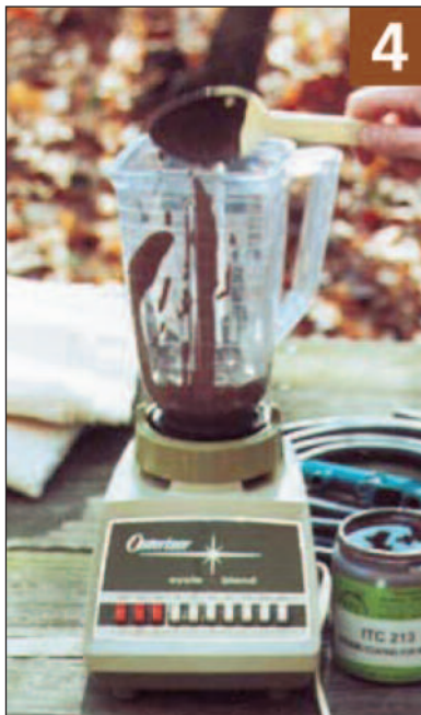
STEP 4 Mix 3 parts of ITC 213 with 1 part water in a blender. Estimate what you need, and make more if necessary or store excess in an airtight container.
