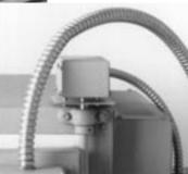
The door cutoff switch turns the elements off when the door is opened, yet the controller remains powered. The switch is housed in the box shown above.
