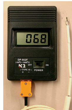
DT-27 Digital Pyrometer (max temp 2000°F)
